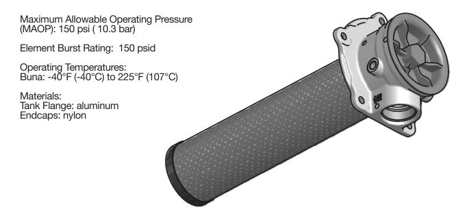
Drawings are for reference only. Contact factory for current version. 1/8-27 PTF 2 PLC'S REF. Ø4.06 3.500-10 BUTTRESS PORT OPTIONS SEE TABLE 2.41 2.70 15/16 (24MM) HEX 941664 TORQUE 200-240 IN-LBS Ø3.33 O-RING THRU. HOLE 6.20± .060 SINGLE 9.79± .060 DOUBLE 2.045 14.55 ± .060 TRIPLE 90 DIA FLAT 5 PLC'S 369 Ø.345 ON A Ø5.50 B.C. 1/8-27 PTF 5 PLC'S 2 PLC'S EQ. SPACED .400 MIN CLEARANCE FROM TANK BOTTOM Ø3.09 **SECTION A-A**
